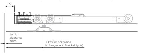
Secure the catch plate body by tightening all 3 screws using a 4mm allen key
