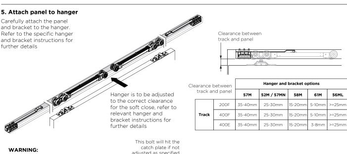
Ensure bolt should NOT extrude to the top surface of hanger, otherwise the bolt will hit the catch plate if not adjusted as specified
